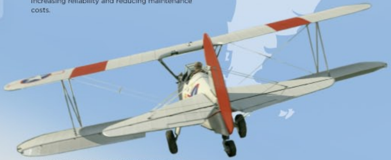
Early aircraft like the Stearman biplane used as a trainer during World War II (above) or the Wright Flyer (1903) pictured below, featured wooden frames with stretched and treated fabric (canvas) to form the outer windproof shell.
